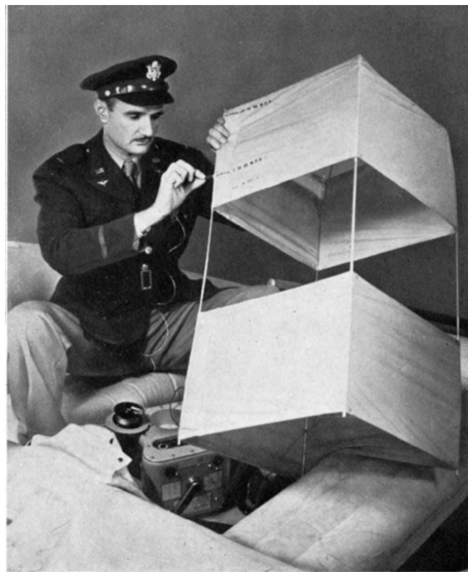
Fig. 12 — Attaching of Antenna to Kite M-277-A
