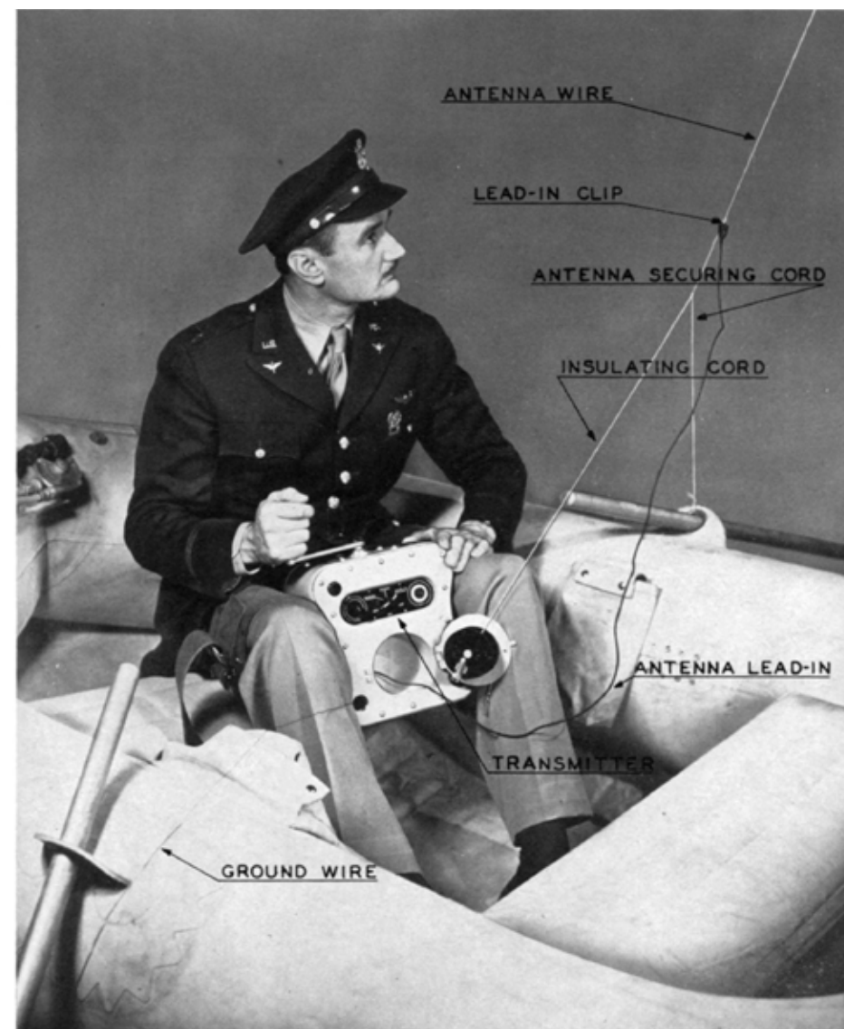
Fig. 9 — Radio Transmitter BC-778-A in Operating Position
